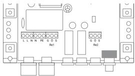
L, N and PE terminals are connected 2 each to facilitate bridges to the relay,
